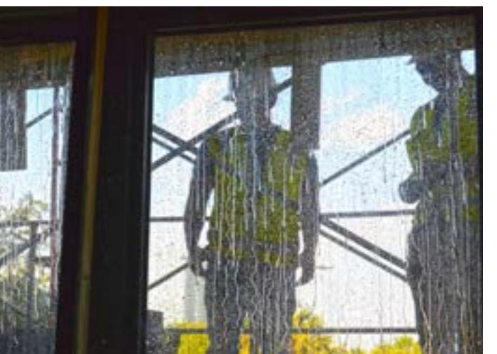
Water resistance tests are performed on specimens to check for water penetration under cyclic and static air pressure. The air pressure is intended to simulate actual natural weather characteristics such as normal and extreme rainstorm with wind events.
