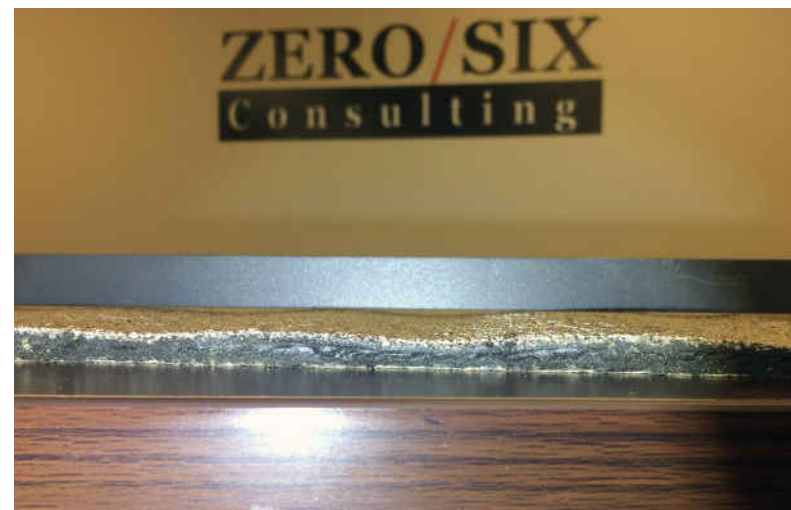
Figure 3: Uneven Distribution of Modified Asphalt beneath Membrane.
