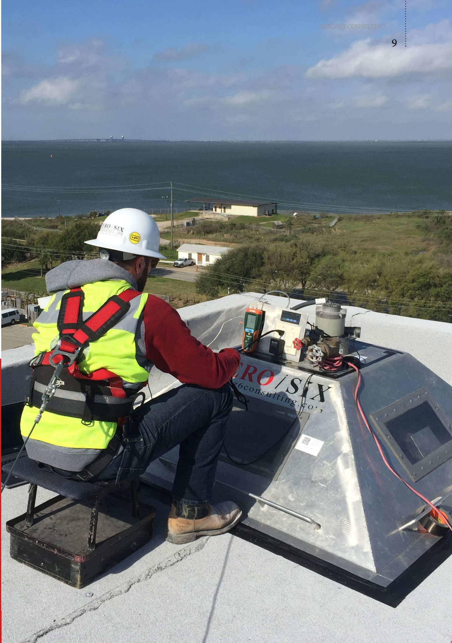
Photo Info : 'Z6 Commissioning performing roof membrane uplift resistance testing
